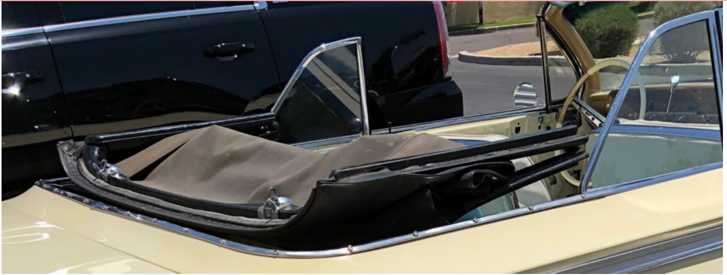
1st TOP INSTALLED DRIVERS SIDE DAMAGE COMPRESSION DAMAGE CAUSED BY FRAME MISALIGNMENT WHILE FOLDING DOWN
