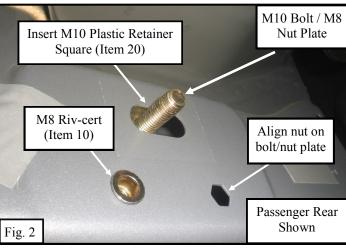
If factory threaded holes are present, do not align the nut on the bolt/nut plate. The threaded hole will be used instead of the nut.
