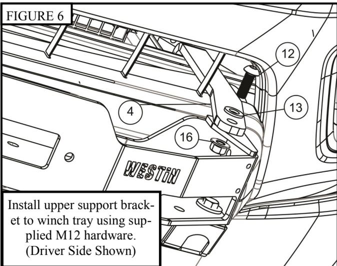
Install upper support bracket to winch tray using supplied M12 hardware. (Driver Side Shown)
