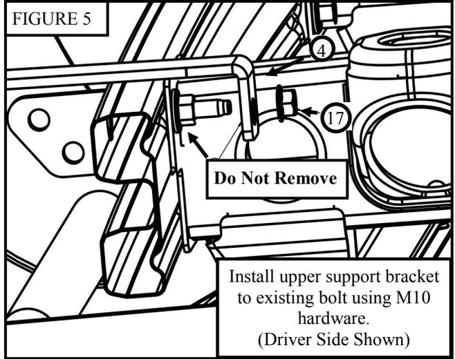
Install upper support bracket to existing bolt using M10 hardware. (Driver Side Shown)
