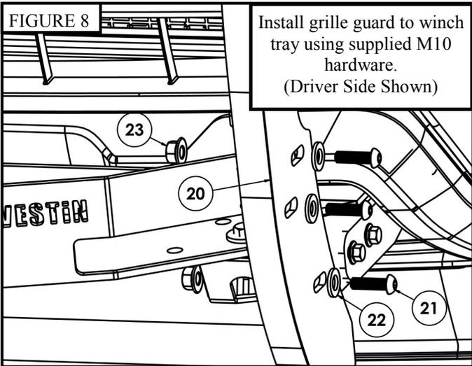
Install grille guard to winch tray using supplied M10 hardware. (Driver Side Shown)
