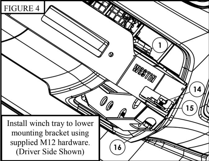
Install winch tray to lower mounting bracket using supplied M12 hardware. (Driver Side Shown)
