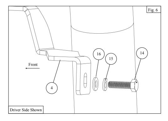
6. With the brackets now in place, loosely install the bull bar using the supplied M8 and M12 hardware. See Figures 7-8.
