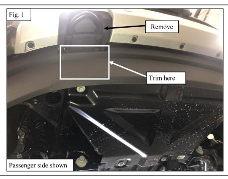
3. Using The supplied M12 hardware (items 6-8), loosely install the mounting brackets (items 2-3) in the tow hook mounting locations. See **Figures 2-3.** Trim front valence as necessary.
