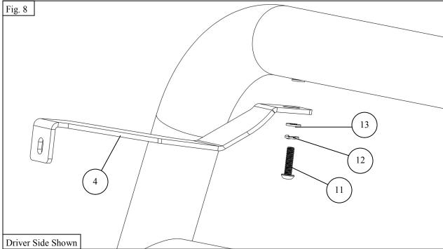
7. Adjust the bull bar as needed and torque all hardware as specified: M8 to 15-18 ft-lbs, M12 to 45-50 ft-lbs.
