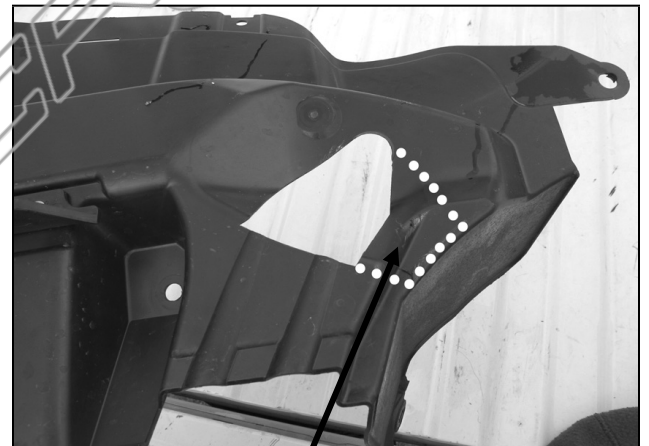
(Fig 2) 07-11 driver side pictured for example only: Cut the plastic splash guard where indicated by the dotted line before installing Sport Bar Brackets
