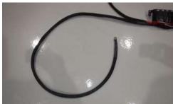
• Before mounting the PDA determine the location of the main power and grounding source. There is a section of black 6 ga wire leading out of the PDA that will need to be connected to a known good ground.
