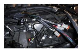
$\bullet$  Try to put the connection in an accessible location in case you need to replace or repair the component.
