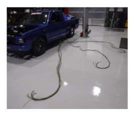
• You do not have to fully remove the harness from the vehicle for sleeving. You can leave the PDA mounted and remove the 3 main branches if desired.
