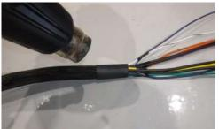
• Secure the taped ends of the sleeving to the harness with heat shrink. The heat shrink should cover the tape and a couple inches on both sides of the tape ring.
