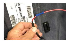
• Double check all connections that you completed by giving a slight tug on both ends of the connection after the heat shrink is complete or the pins and connectors have been installed. The goal on installing the harness is to complete this process with a clean and secure attachment of all wiring connections, making sure they are not subject to damage due to heat or moving parts.
