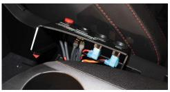
• A detailed color wire identification and connection chart and full color diagram have been provided with the harness to ensure proper connections. Follow these steps and chart to complete all component connections.
