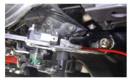
• The solid red 16ga wire is for applications using a wide-open throttle switch instead of a TPS signal. This will connect power to the wide-open throttle switch. This wire can connect to the red/white 12v keyed hot wire or connect to a fuse tap in the fuse box.
