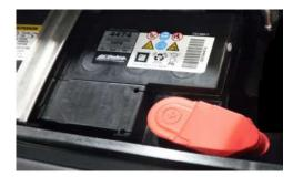
• We recommend connecting the main power supply wire and the main ground wire directly to the positive and negative post on the battery. However connecting to the power point junction box and a known good ground point in the engine bay will be ok.
