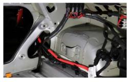
• After you have completed sleeving and heat shrink for each lead, reinstall the harness in its permanent mounting place.
