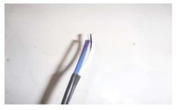
• At the end of each lead, use a piece of tape to tightly group the wire ends so that the sleeving will easily slide over.
