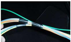
• After all branch outs have been taped, remove the harness from the mounting locations to begin the sleeving process.
