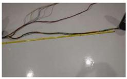
• To cut a specific length of sleeving, begin with one of the harness branches closest to the PDA and measure up to the next branch. Make sure to add 6 to 8 inches to the measured length due to the fact that the sleeving will shorten as it expands over the harness.
