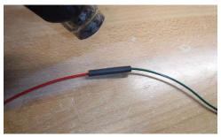
• In some cases, you may not be using a connector, but simply attaching the two wires. When you are mating the two wires together, we recommend you solder the connections and protect them with the provided glue shrink.
