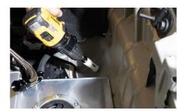
• In the event that the harness needs to route through a drilled hole in the firewall use the supplied grommets to protect the wires from being damaged.
