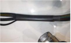
• Using heat shrink, cover the breakout or the branch off to ensure you have no exposed wires. This length will need to cover the end of the sleeving on the first section of wires to the start of the sleeving on the next section of the harness.
