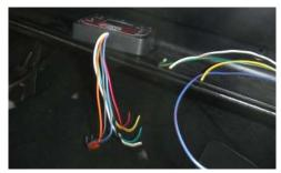
• The wires in each section of the harness will have several component leads that terminate in different destinations. Make sure when mounting a harness lead that you are properly securing it so it is avoiding any extreme heat or any moving parts that can damage the harness.
