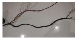
• Slide the sleeving to the measured section of the harness. Evenly distribute the sleeving along this section of the harness in both directions until it has fully expanded.
