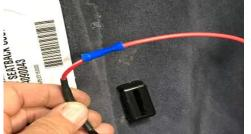
• The red/white 14 ga wire will be used to connect the keyed hot power source for each switch on the switch panel. This connection is specific to each vehicle. In most cases a fuse tap with the appropriate amperage can be used and connected in your vehicle's fuse box. For recommended connection location for your specific vehicle please visit the Nitrous Outlet website Technical Support tab for our Pin-Out Reference Charts.
