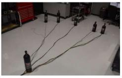
• With the harness out of the vehicle, stretch it to full length.
