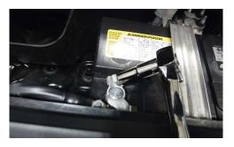
• Connect the black 6ga wire leading out of the PDA to the negative battery terminal or a known good ground.
