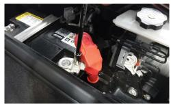
• Connect the red 6ga wire to the positive battery terminal or positive voltage supply.
