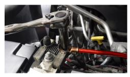
• Reconnect the battery cables, include the wiring harness ground and power wires.
