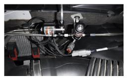
• Once your engine compartment components are installed, connect the harness to the system and purge solenoids. Each lead of the harness is labeled and terminated for the attaching component. Connector installation instructions are located on page 5 of these instructions. The solenoid wires can be installed into either side of the Deutsch connector. Make certain when installing the harness it is free from any extreme heat sources or moving parts that can damage the harness.
