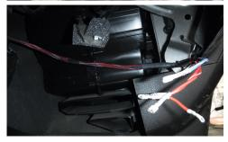
• Route the switch panel wiring to the cabin of the vehicle. You may need to drill a 9/16" hole and use the provided grommet for this step.
