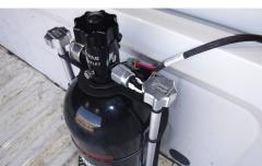
• Connect the bottle heater and nitrous pressure switch leads.
