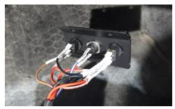
• Once all of your leads are plugged in to the under hood and bottle components, move to the interior and connect the switch panel leads at the switch panel. Follow the wire identification chart provided in the wiring schematics for the proper connection of your leads.
