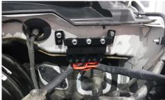
• This harness is designed for the relay center to mount under the hood, close to the battery for positive and negative connections. Applications that have the battery in the rear of the vehicle will require connection to the positive terminal and known ground terminal or stud under the hood.
