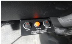
• Install the switch panel in your vehicle. The bolt holes in the switch panel are designed for #10 mounting hardware.
