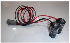
• If you have a system that includes a nitrous and fuel solenoid, connect the nitrous and fuel solenoid leads into the same connector. Make sure to have one wire from each solenoid in one side of the connector and the remaining wire from each solenoid in the other side of the connector. Connector installation instructions are located on page 5 of these instructions. Make certain when installing the harness it is free from any extreme heat sources or moving parts that can damage the harness.
