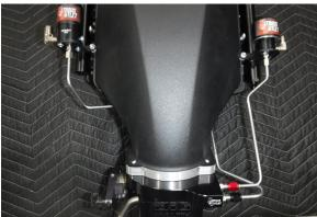
**Step 14:** Repeat the same steps to install the nitrous hardline.
