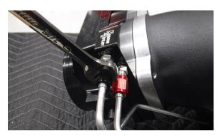
**Step 16:** Using a 7/16" wrench, tighten the compression and b-nuts on each hardline.
