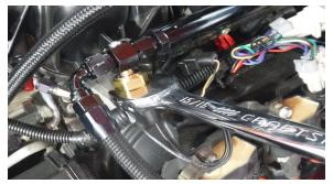
The in-line manifold can be installed directly to the fuel rail.
