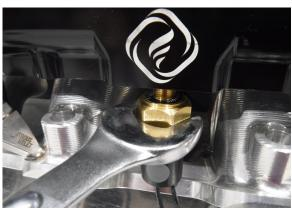
The switch can also be installed directly to the fuel rail provided it has a 1/8" NPT port.
