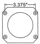
This kit is for axles with a 3 3/8" spread center to center on the top two bolt holes (pictured left). If your axle flange measures 3 1/8" from center to center, you need our kit AFXRD01, AFXRD05, AFXRD06 or AFXRD07. Call 800.405.2000 for further assistance.
