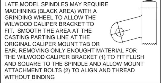
Figure 3. Machining Diagram
