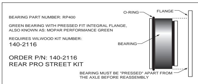
Figure 1. Press Fit Flange Bearing Configuration
