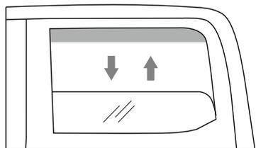
6. Raise the window until it touches the deflector. Carefully pulling the deflector outwards, roll up the window with abrupt movements. Repeat this action 4-5 times, then leave the window closed.
