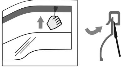
8. To ensure better installation of the deflector and better adhesion between the tape and the surface of the rubber seal, it is strongly recommended that you use the plastic blade, moving it slowly between the window's inner rubber seal and the deflector.
