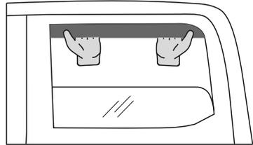
4. Immediately after installing the deflector, adjust its position by carefully pulling it outwards.
