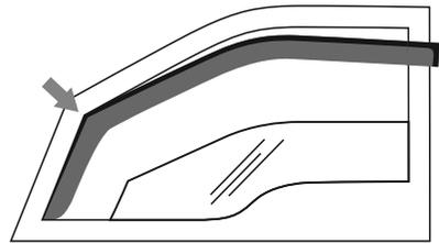
4. Shift the deflector forward, fitting the deflector frame into the channel completely. Make sure the deflector is placed above the lower window frame.
