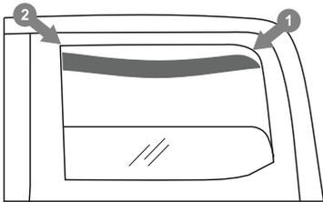
3. The deflector must be installed starting at the back. To do so, place the back part of the deflector frame into the channel and move the front part upwards. Position the entire deflector frame into the window channel, placing the frame between the fastening brackets and the rubber seal as is shown in the picture.
