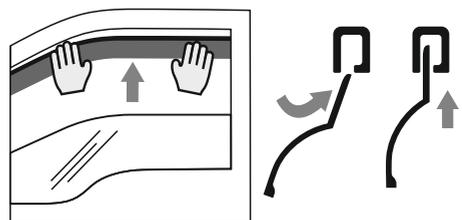
6. Starting with the front part of the deflector, insert it into the window channel.
