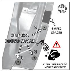
**FIGURE D** Gently bend bottom of BMF52-LF/RF to conform to wheel well. Place bolt-end of bracket over logo-side of flap through mount 1.
