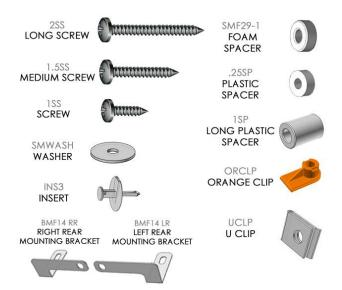
**Recommended Tools** Low-profile offset or ratcheting screw driver, 7/16<sup>th</sup>" wrench, flathead screwdriver. **Important Tips** Installation should be done on an even surface. Do not use power tools to tighten hardware. Hand tools only. Avoid overtightening.
