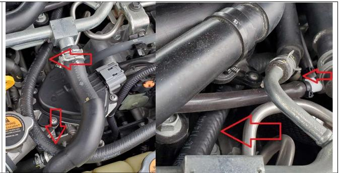
7 Lubricate hose ends and make connections to J&L oil separator. Reinstall engine cover.
