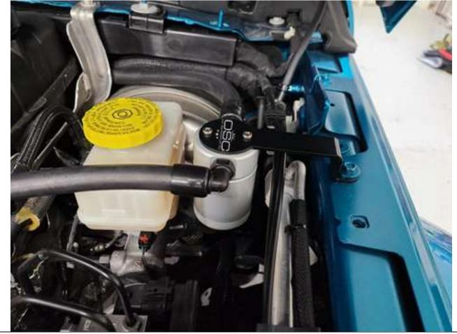
**4xe owners-** You will need to remove the black plastic bracket that is holding two small wiring harnesses. Pull harness pins out of bracket with clip pry tool. Secure two small harnesses to large orange wire with supplied ziptie. You will mount the J&L Bracket with the bolt that was closest to the rear of the vehicle.
