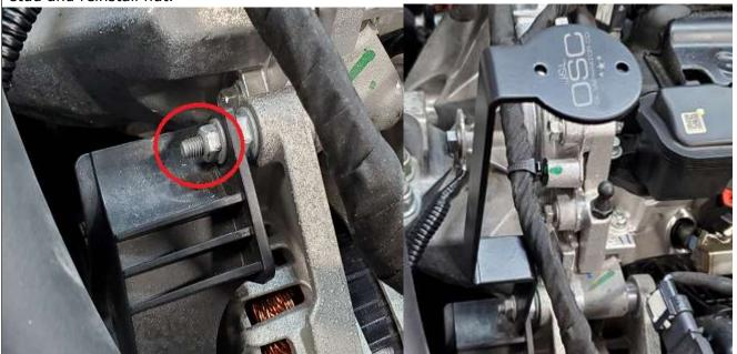
Mount J&L Oil Separator to mounting bracket with supplied mounting screws
