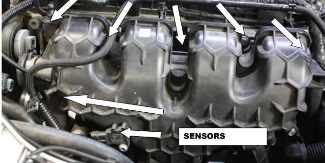
Page 1 of 4 11-08-22 Pull manifold back and shine a light behind to see from passenger side. Remove PCV line from the intake to the block.
