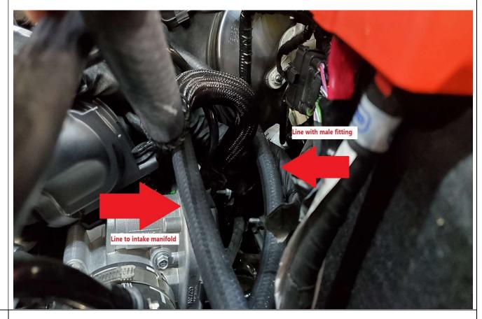
Note: The fitting in the J&L Hose has a push button release, along with a locking tab. See below for how this fitting operates. The locking tab can only be engaged once installed onto connection.
