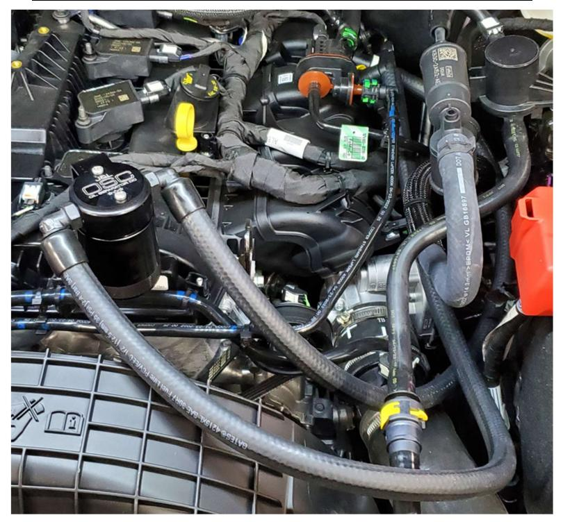
Check oil separator after 1000 miles of driving to assess how much contaminates your engine is putting through the PCV system.
