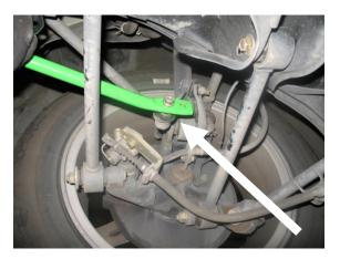
**9.** Thoroughly lubricate the **inside** of your new bushings using the supplied grease. Place the bushing on the new Anti-Sway Bar. Refer to the original equipment Anti-Sway Bar as to the proper bushing location.
