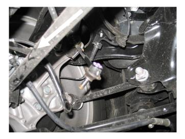
7. Remove the factory Anti-Sway Bar by removing the factory bushing brackets.
