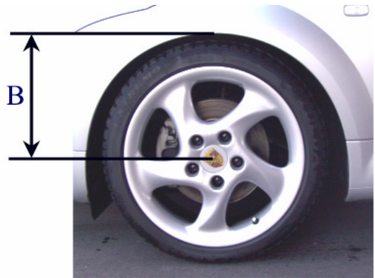
Measurement B Wheel hub center wheel arch
