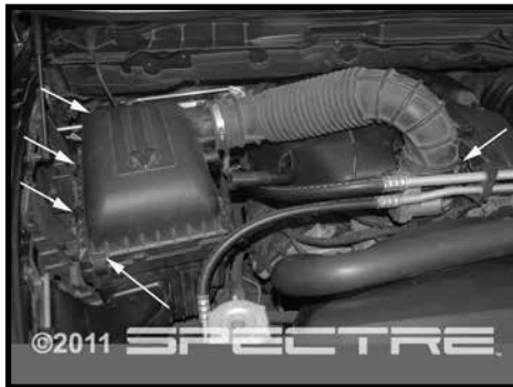
Step 4 Loosen the clamp on the tube going to the throttle body. Unclip the four hold down clips on the air filter lid. Remove the intake tube and airbox lid assembly from the vehicle. Remove the stock airfilter.
