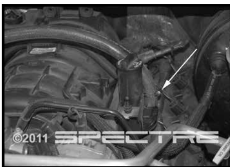
Step 7 Install the new PCV breather line supplied in the kit. Once in place securely fasten with clamp provided.
