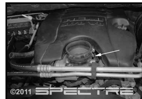
Step 9 Install the coupler onto the throttle body. Tighten the clamp on the throttle side and make sure the intake side clamp is installed but left loose.
