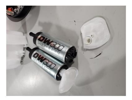
4 – Shorten the supplied wiring harness to approx. 8-inch (205mm) and crimp on the supplied ring terminals. Attach both ground wires to the pump negative terminal and attach each pump power wire to its separate positive terminal. Tuck the remaining wire into the cavity provided above the pumps.
