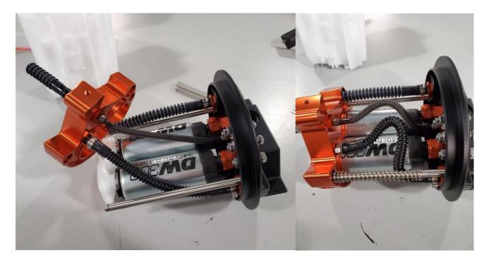
10 – Remove the plastic connector and strip the ends of the provided fuel level sending unit wiring and crimp on the provided ring terminals, it may be necessary to double the wire over due to its small size. Attach the level sending unit wiring to the Level positive and negative terminals.
