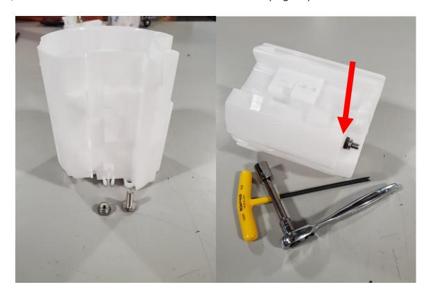
6 – Assemble and install the rubber one way valve into the bottom of the bucket. Once it snaps into place it should pivot freely.
