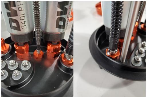
8 – Using the remainder of 5/16" hose from Step 2, cut it down to 2-2.25" (50-57mm) and attach it to the single 5/16" hose barb fitting on the bottom side of the orange center plate, secure with a 5/16" clamp.
