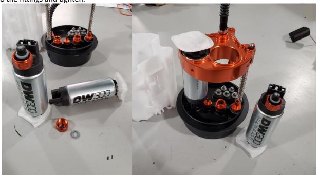
2 – Install the supplied longer 10" x 5/16" convoluted tube onto the return fitting and secure with the supplied 5/16" pinch clamp. Slide the center plate over the pumps and return tube, reinstall the e-clips, cut the return hose flush with the bottom of the return plate when its fully extended.
