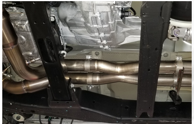
Detail 17: Catback connection (shown with SW catback)
