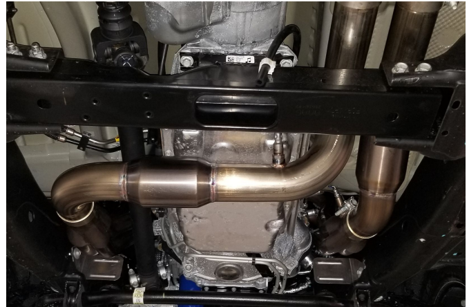
Detail 16: Headers and leads installed
