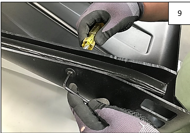
Slide another supplied 6mm Washer onto the back of the screw from the inside of the Roof. Install a supplied 6mm-1.0 Nylock Nut onto the back of each Screw. Tighten with a 4mm hex key on screw side and a 10mm socket over Nut.
