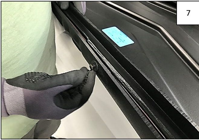
Place Screw/Washer combo through each hole Roof and Adapter.
