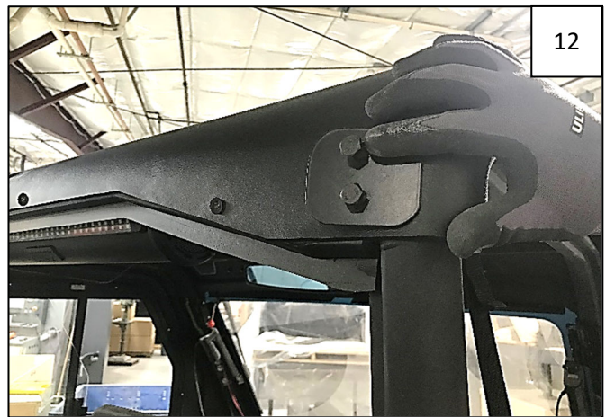
Place a supplied Bracket over feature, aligning holes with factory holes in frame. Install 2 supplied 13mm Hex Bolts through holes in Bracket and into factory holes in frame (both sides).
