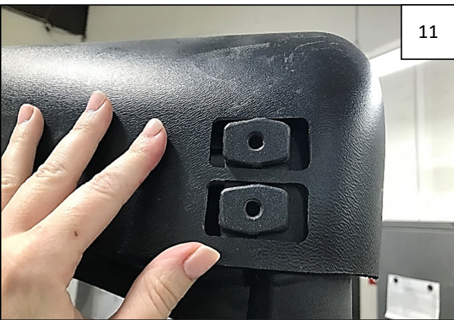
At rear of frame, align holes in UTV roof with feature shown, one on either side of frame.
