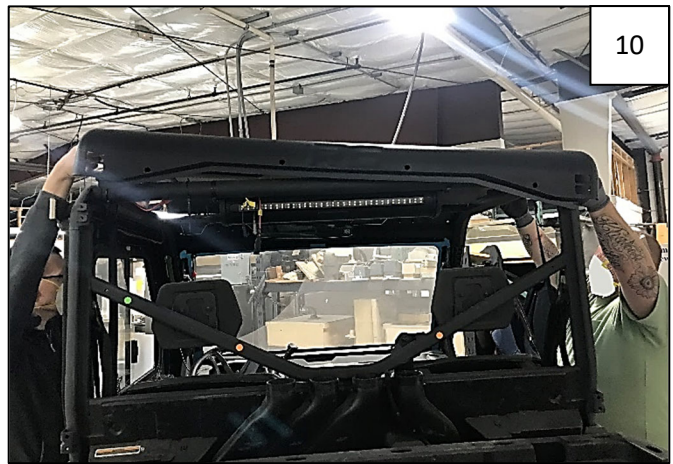
Slide Roof over top of UTV frame.
