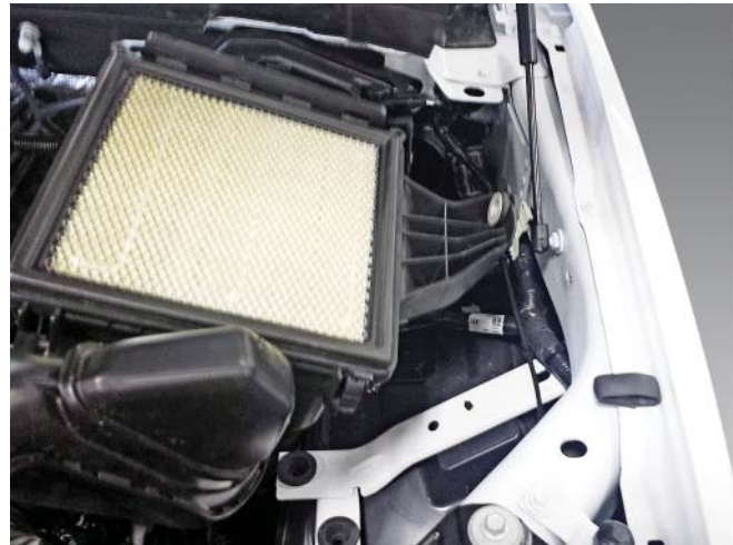
11. Remove the self-tapping screw retaining the dirty air inlet onto the lower air box.
