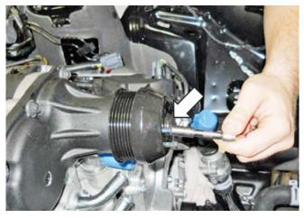
Re-install the FEAD belt on the supercharger by rotating the tensioner clockwise and routing the belt as shown in the routing below.
