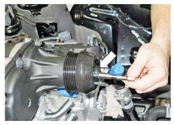
Remove the belt from the supercharger by rotating the tensioner counterclockwise and removing the FEAD belt from the supercharger pulley. Then remove the supercharger pulley.
