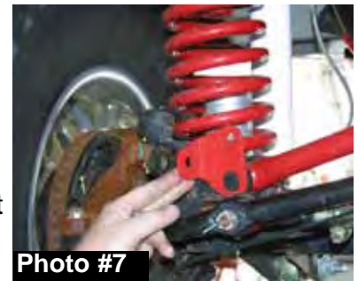
5/16" x 3/4" thread cutter flange bolt.
