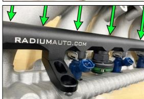
8. As shown, slide a phenolic washer under each mounting foot.
