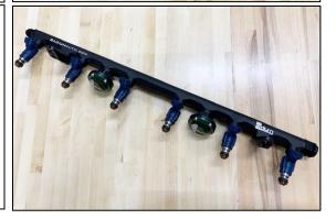
5. If reusing stock or OEM compatible fuel injectors, slide the OEM clips on locking the injectors to the fuel rail.
