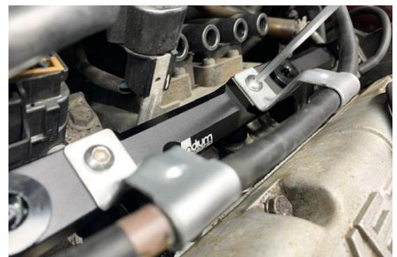
25. After everything is reinstalled in a reverse order, cycle the key a few times (without starting engine). This allows the fuel pump to prime the system.
