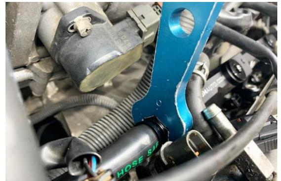
24. Position the cable bracket stays 180 degree from how they were oriented with the OEM fuel rail. The single cable bracket variation is shown. The early dual cable bracket variation will slightly differ.
