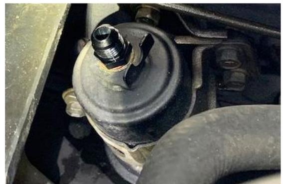
15. Install fittings to the 4 ports. Lubricate all O-rings prior to securing.
