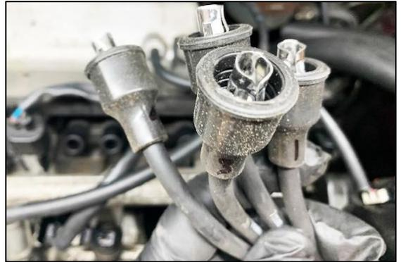
8. Gently pry the cable(s) from the fuel rail stays. NOTE: The first 4G63 engine variations will have 2 cables.
