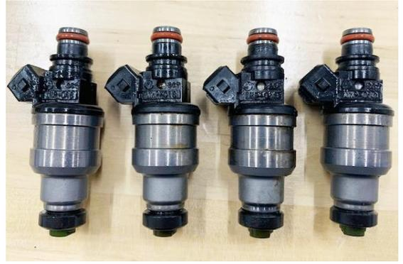
11. Press the 4 fuel injectors back into the lower ports on the cylinder head.
