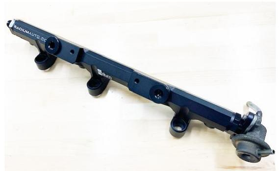
16. Lubricate the fuel rail injector ports.
