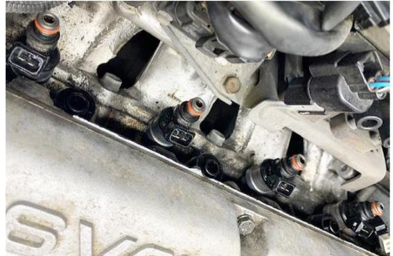
12. When installing the 3 mounting feet to the fuel rail, apply a high strength thread locker to the six M5x0.8mm bolt threads. Secure using a 4mm Allen wrench.
