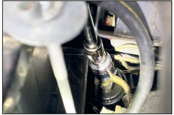
6. Using pliers, remove the return hose from the fuel pressure regulator. Catch any fuel that may spill from this connection and properly dispose.
