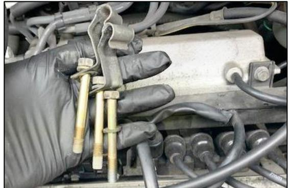
9. Carefully pull the fuel rail upwards away from the cylinder head. Be careful not to lose the 3 OEM insulating spacers.
