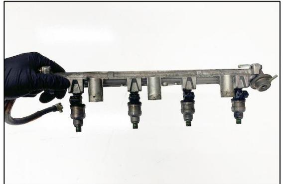
10. Be sure to find the lower injector O-rings as they will sometimes get stuck in the cylinder head. Inspect the condition of both the upper and lower injector O-rings and replace if necessary.
