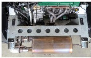
E. Line up the larger hole in the shims with the threaded holes in frame. Make a mark on the frame at the smaller countersink shim holes with pen. Repeat this process at all four locations.
