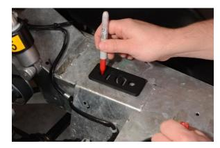
F. Use a 1/4" drill bit and drill holes at the locations marked with the pen.
