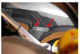
A. Locate the factory clamshell shims that are taped to the rear chassis structure. Completely remove the tape and the shims at all four locations. These will not be reused.
