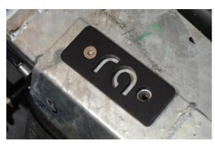
H. Reach your hand, or use a long wrench or two wrenches taped together, into the frame rail and install one of the included lock nuts to the bolt inserted in the previous step. Tighten the bolt. This should now be done at all four locations.
