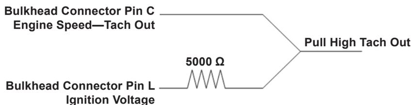
**NOTE: When connected to the CP Supermatic Connect and Cruise Harness the pull up resistor is not required for the Transmission Controller.**
