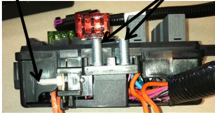
Attach a 12 volt ignition switch feed from the vehicle to the pink ignition switch wire in the harness (this is required to enable the proper power-up sequence of the ECM). This can be routed into the passenger compartment with the accelerator pedal connector and diagnostic link connector. Next, connect battery power (minimum 8 gauge wire) to the horizontal stud on the fuse relay center. The other two studs are for accessories and are 50 amp fused. The harness installation is complete.
