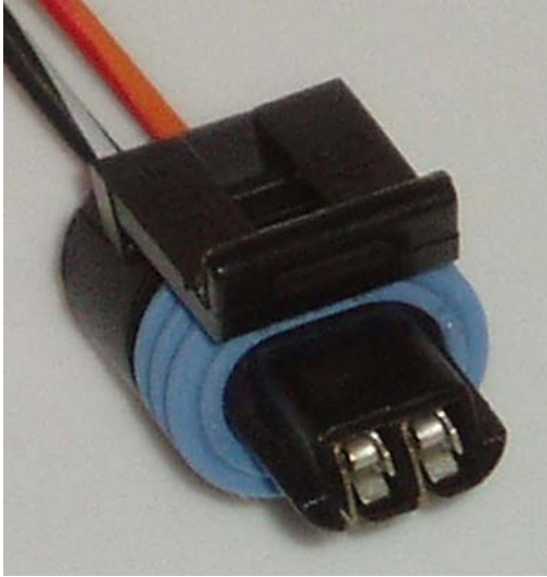
Figure 2. GM 4L60E VSS connector
