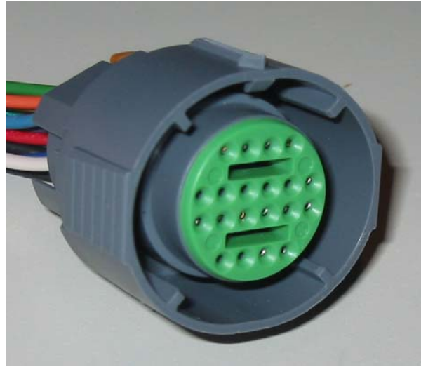
Figure 3. GM 4L60E main connector
