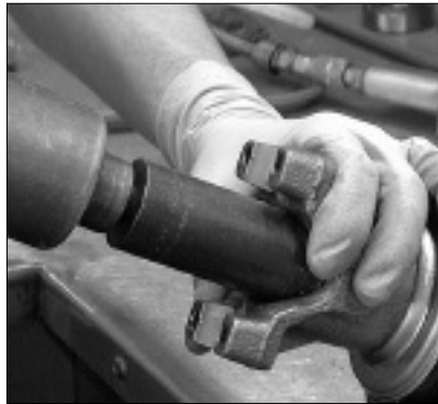
1/2" impact gun on pinion nut
