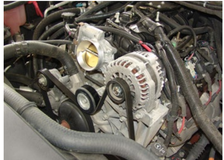
Throttle Body Inlet Tube Removed
