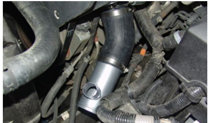
Rubber 45° Elbow With Bypass Tube
