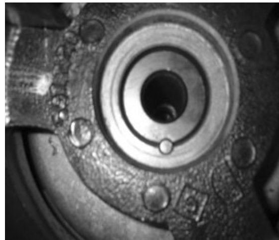
Harmonic Balancer Pinned to Crankshaft
