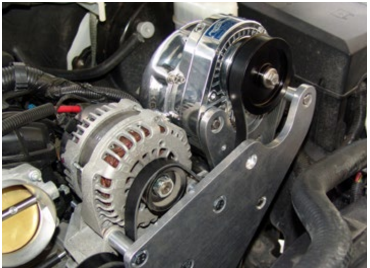
Sub-Bracket Assembly Installed
