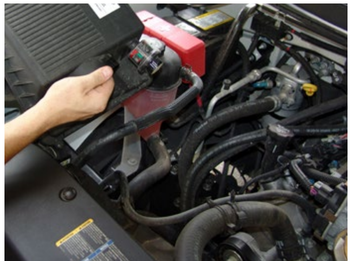
Air Filter Box
