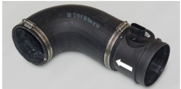
MAF Sensor Installed On Rubber 90° Elbow
