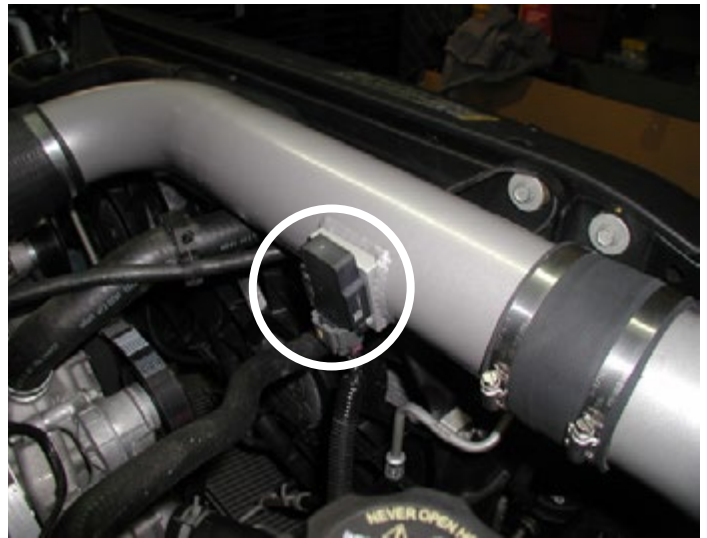
MAF Sensor Installed
