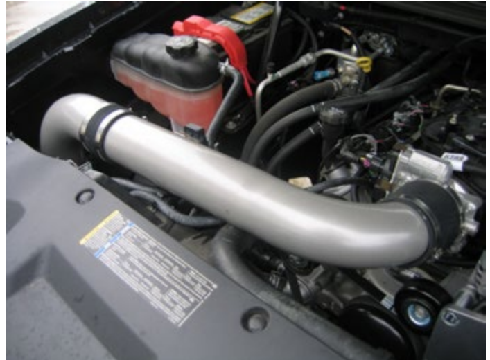
Steel 90° Elbow Mounted To Upper Tube
