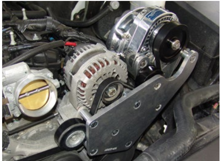
Serpentine Belt Installed
