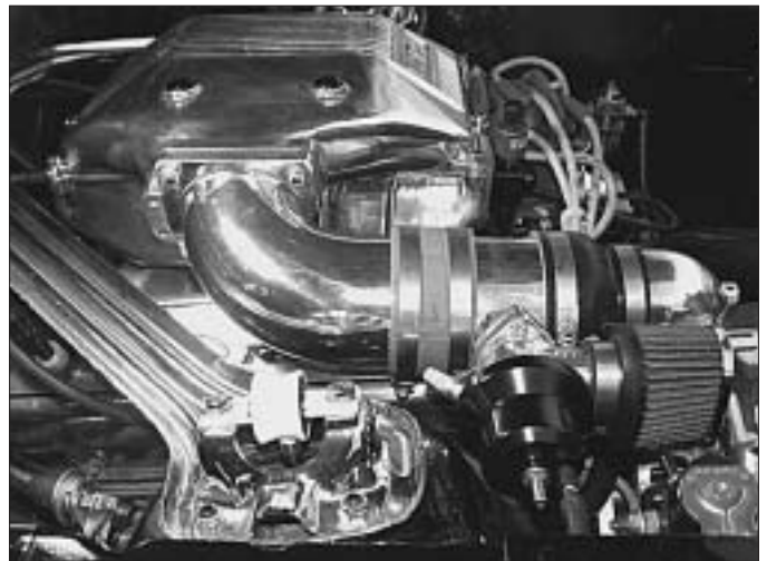
Fig 9-c / Passenger side discharge duct. (1969 351 Mustang)
