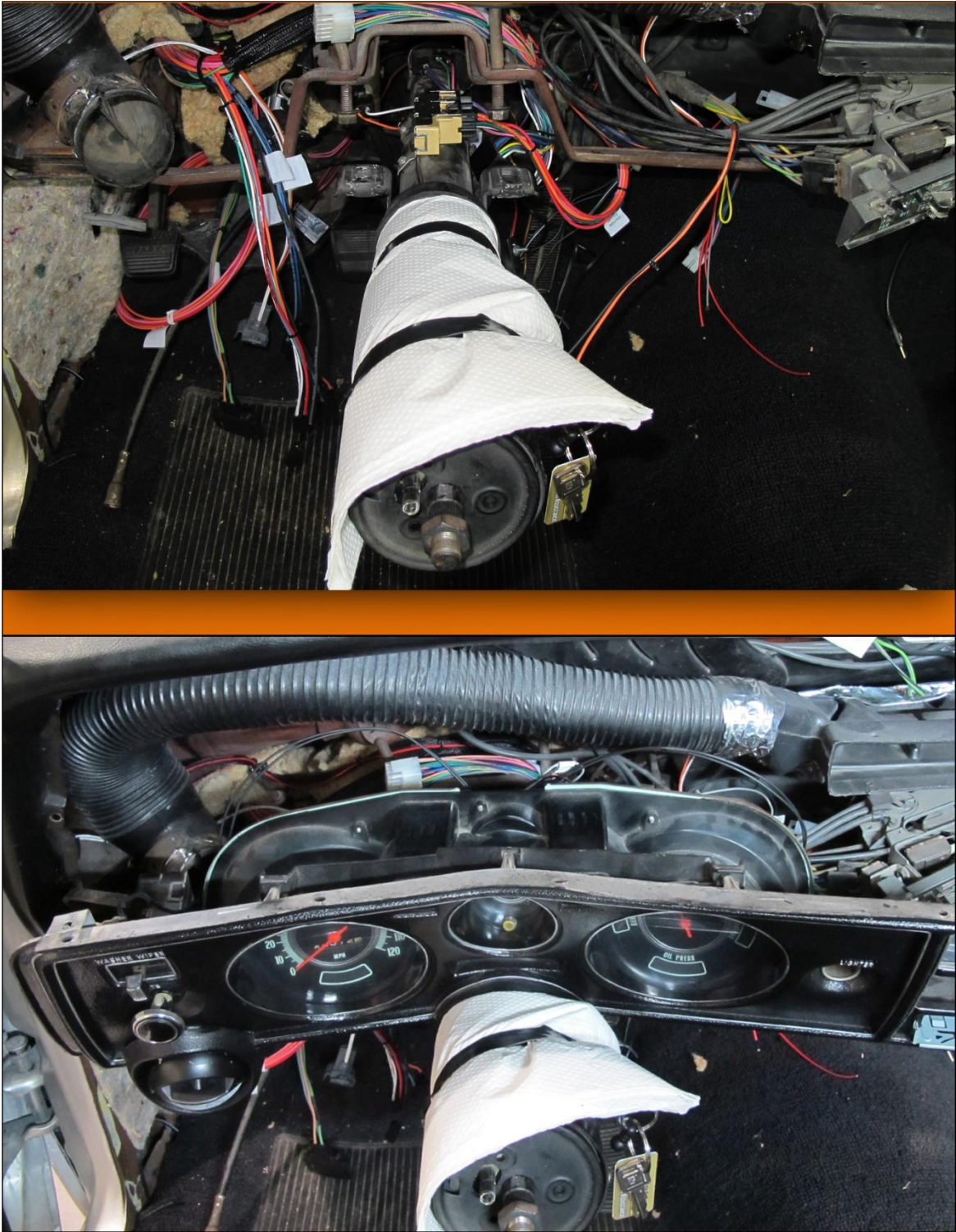
The above photo is of a 1969 model dash, which is why the gauge cluster and connection on the top of the column look different from your 1968.
