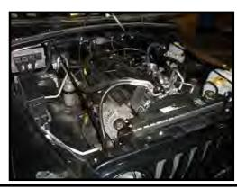
2. Remove 4 bolts that fasten the throttle body to the intake manifold. Lift throttle body and remove gasket. Install Throttle Body Spacer in between throttle body and intake manifold, using supplied longer bolts. Install supplied gaskets between intake manifold and throttle body spacer, and between throttle body spacer and throttle body. Torque bolts to 23 Nm (200 in. lbs.)
