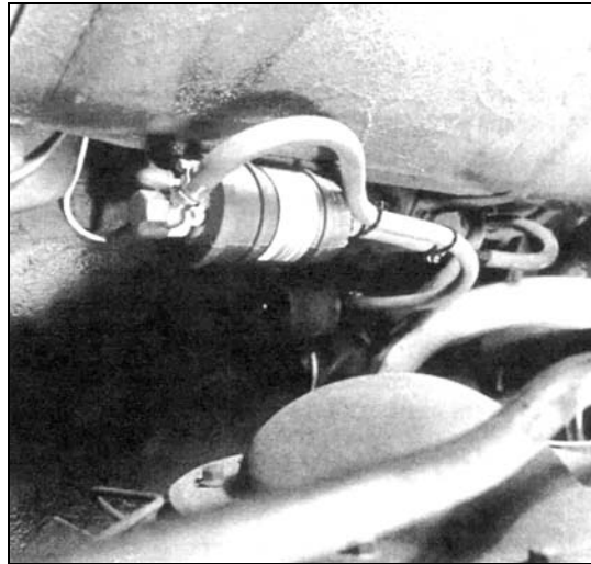
Figure 12 Kit Number 0015NOS Fuel Pump Mounting Location
