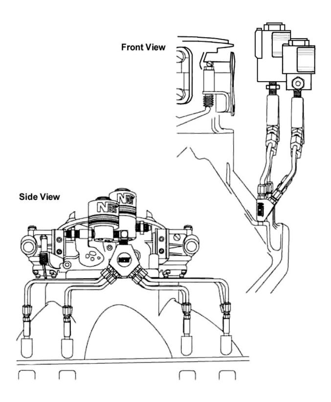
Figure 3 Kit Numbers 04462NOS & 04463NOS Shown Installed—Configuration Two
