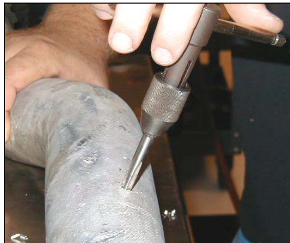
Figure 7 Tap with supplied 1/16 NPT tap.
