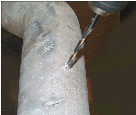
Figure 6 Drill using a 1/4 inch bit.
