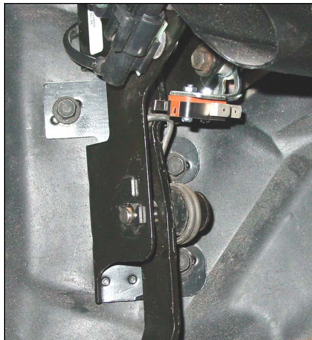
Figure 16 Microswitch in completed location
