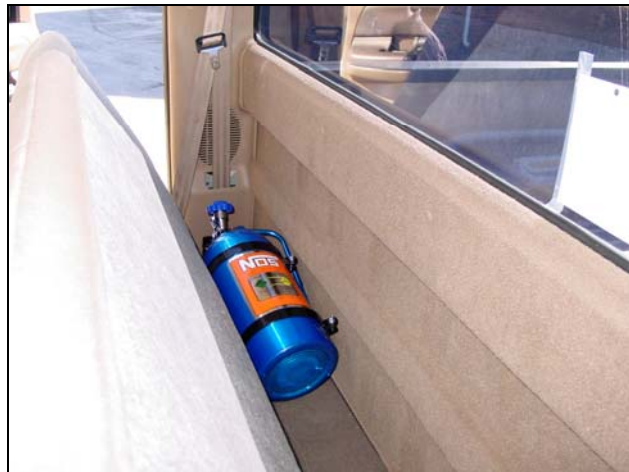
Figure 4 Bottle with blow down tube installed
