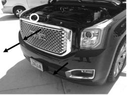
Unclip wiring harness, Location indicated by circle. Remove bumper and grille assembly from vehicle. Lay in a safe location. Grille does not need to be removed from bumper to finish the installation.
