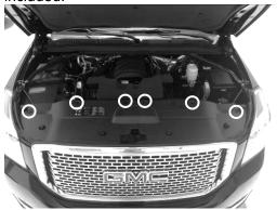
2. Open hood, remove plastic cover by removing 6 retaining clips with flat head screw driver. Locations shown above. Set aside retaining clips and cover.
