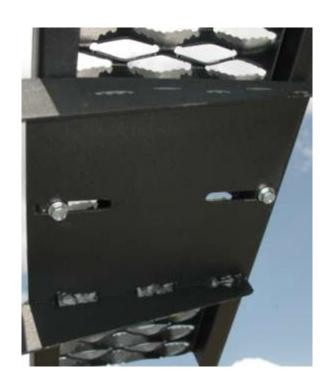
Place the running board on the brackets and install the self tapping screws through the bracket and into the strut flanges as shown in photo.
