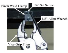
At each mark mount the pinch weld clamp, then by tightening the set screws with 1/8" Allen wrench holding with pair of vise grips for leverage
