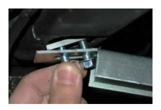
Place (2) 5/16" x 3/4" bolt through CB90 top slot and thread into re-enforcement nut slide nut into hole in frame.
