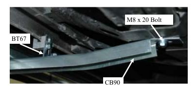
Place 5/16" x 3/4" bolt through BT67 and thread into pinch weld clamp. **Leave loose for later adjustment.** Then place 5/16" x 3/4" bolt through the bottom hole of the BT67 and through the slot in the CB90 put a 5/16" nut onto threads and tighten.
