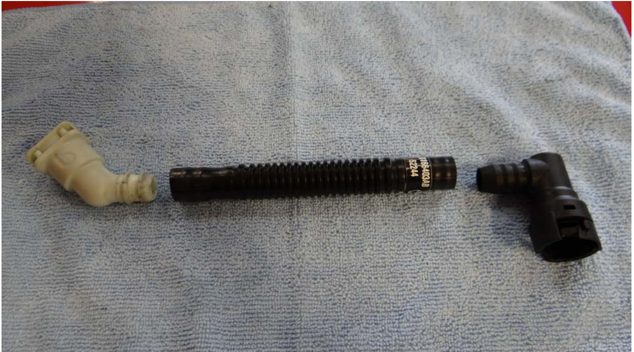
Step 4: Using a razor blade slice PCV line and remove fittings as shown.
