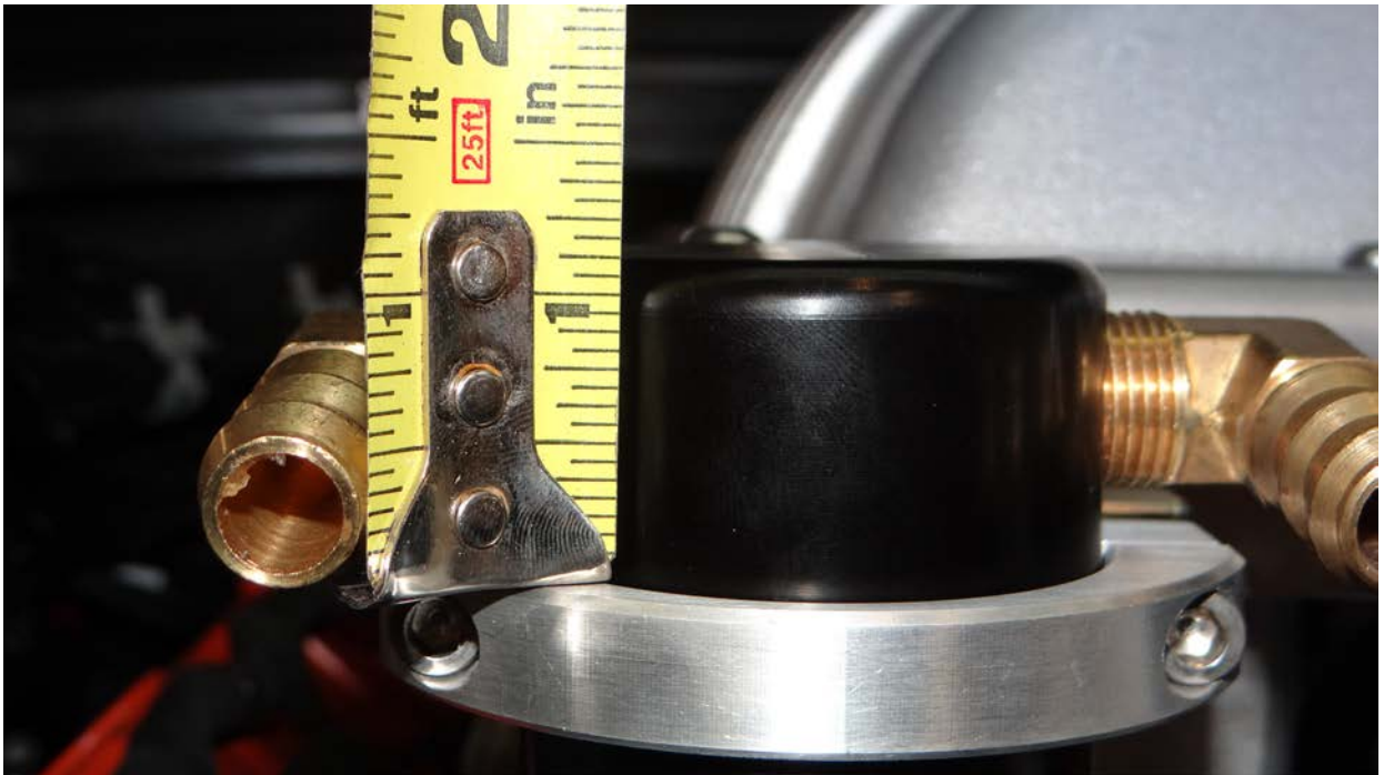
Step 14: Set height to 1"-1 1/8" and tighten billet clamp.
