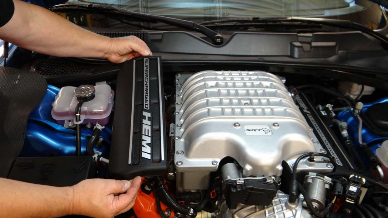
Step 1: Remove engine cover as shown.
