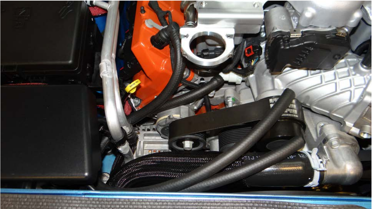
Step 12: Re-install 90 degree fitting to valve cover and re-install 45 degree fitting to intake manifold and route hoses as shown.
