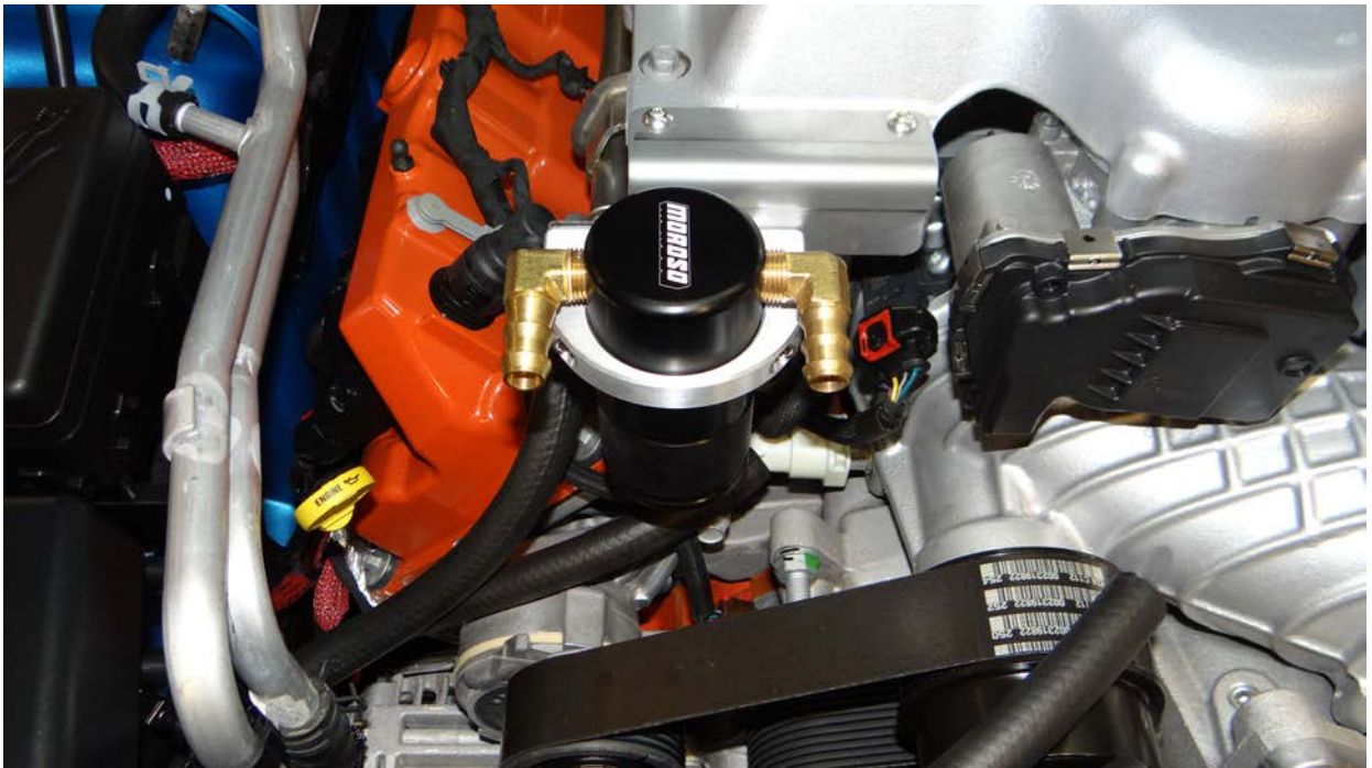
Step 14: Set height to 1"-1 1/8" and tighten billet clamp.
