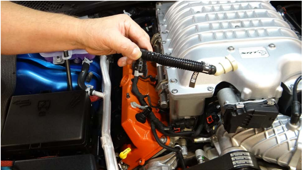
Step 3: Remove PCV line from vehicle.
