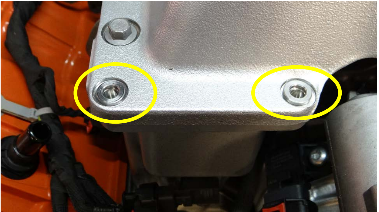
Step 8: Install (2) spacers provided in kit.
