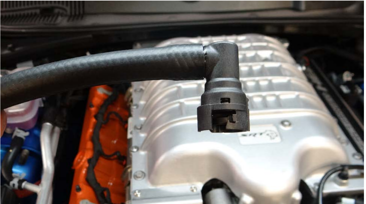
Step 6: Insert 90 degree fitting into one end of 2 nd hose provided in kit.
