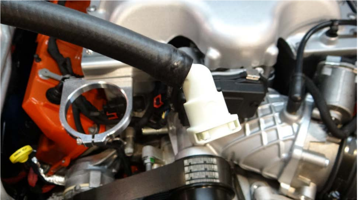
Step 5: Insert 45 degree fitting into one end of hose provided in kit.
