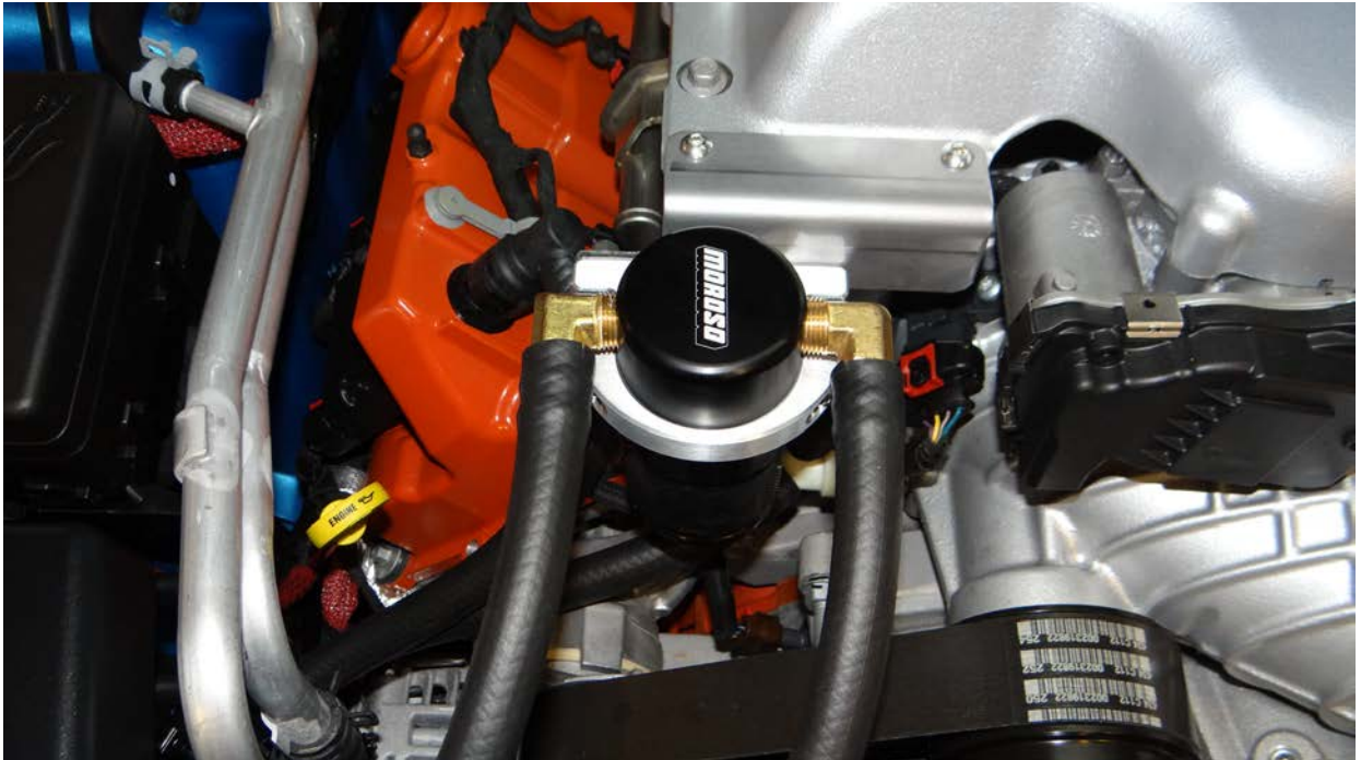
Step 15: Trim hoses as needed and install to air oil separator.
