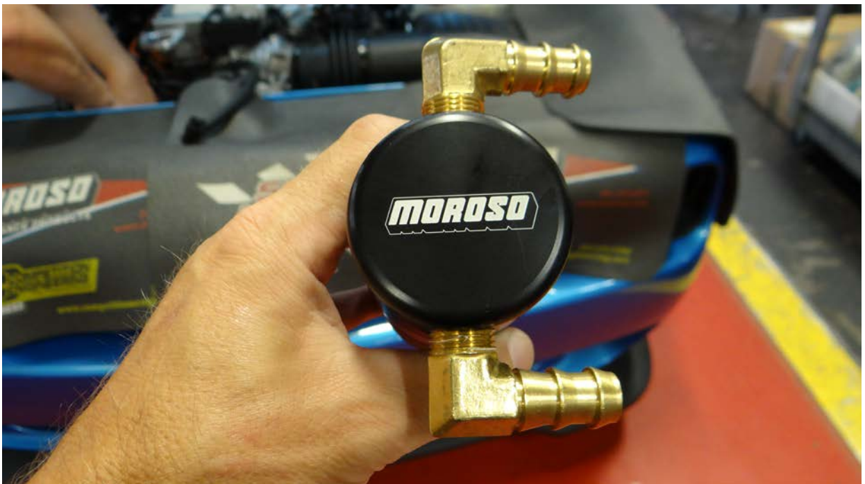
Step 11: Assemble air oil separator as shown using Teflon tape on all fittings.
