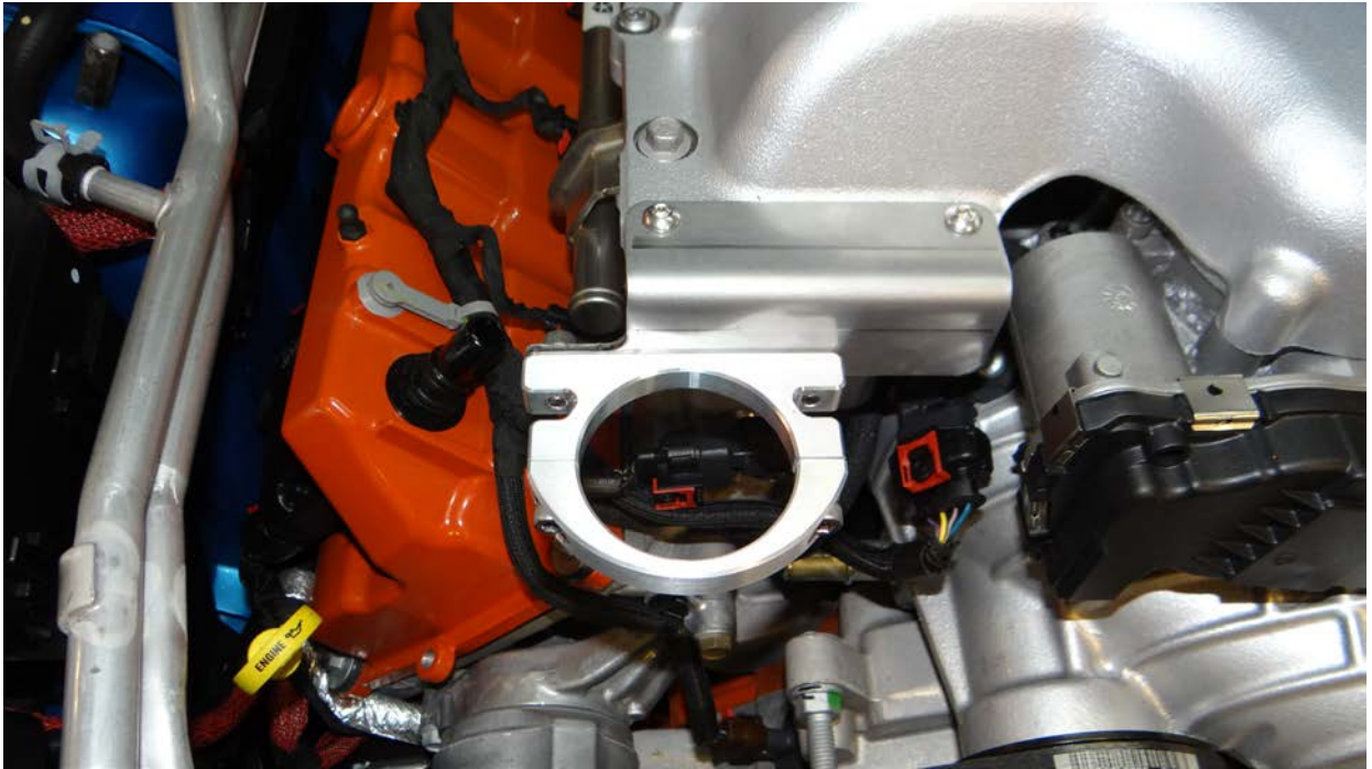
Step 10: Assemble mounting bracket as shown using (2) M6x25mm .
