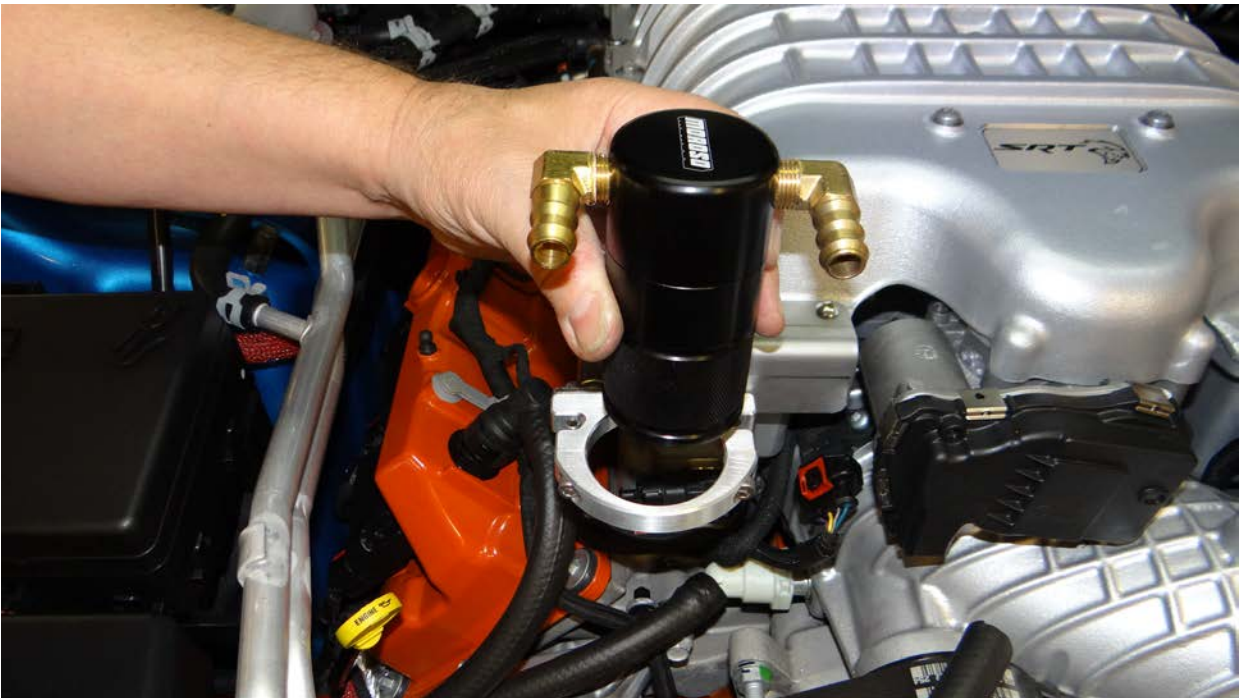
Step 13: Insert air oil separator into billet clamp.
