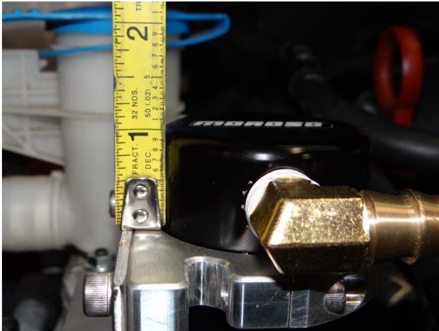
Step 16: Set height to 1"–1 1/8" and tighten clamp.
