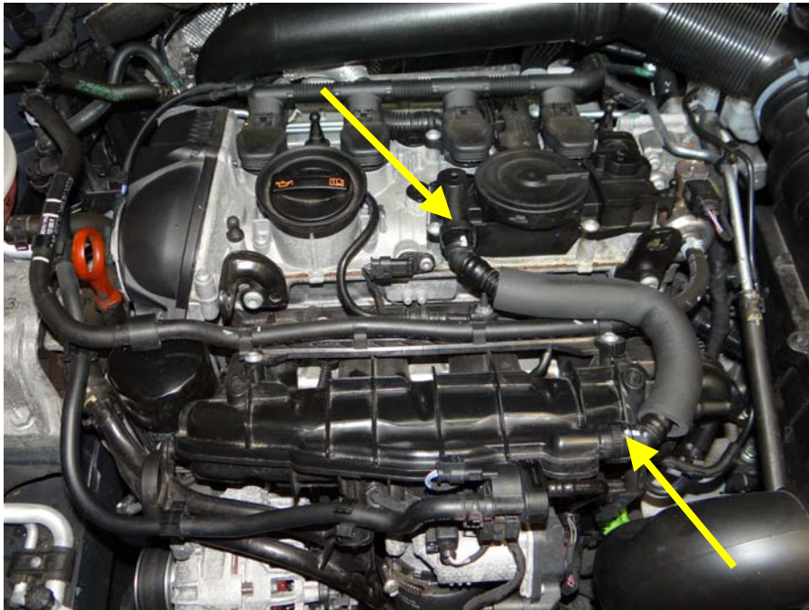
Step 2: Locate and remove PCV line.
