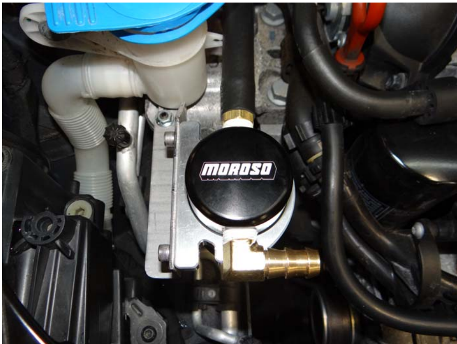
Step 17: Install hoses to Air Oil separator, trimming of hoses will be required.
