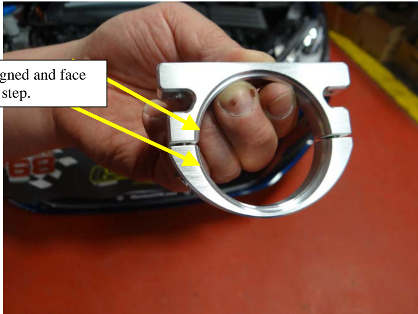
Step 11: Assemble clamp saddle to billet clamp using (2) \frac{1}{4} -20x5/8 SHCS. Do not tighten.
