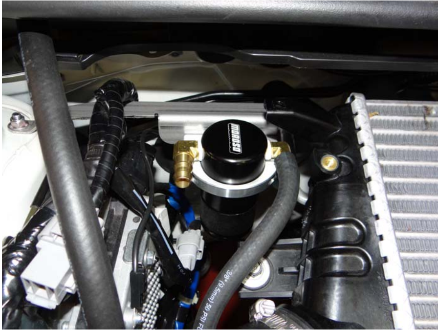
Step 16: Install hoses to Air Oil Separator, trimming of hoses will be required.
