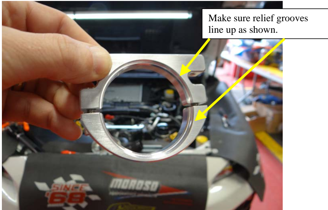
Step 10: Assemble billet clamp to billet saddle using (2) 1/4-20x5/8 SHCS. Do not tighten.
