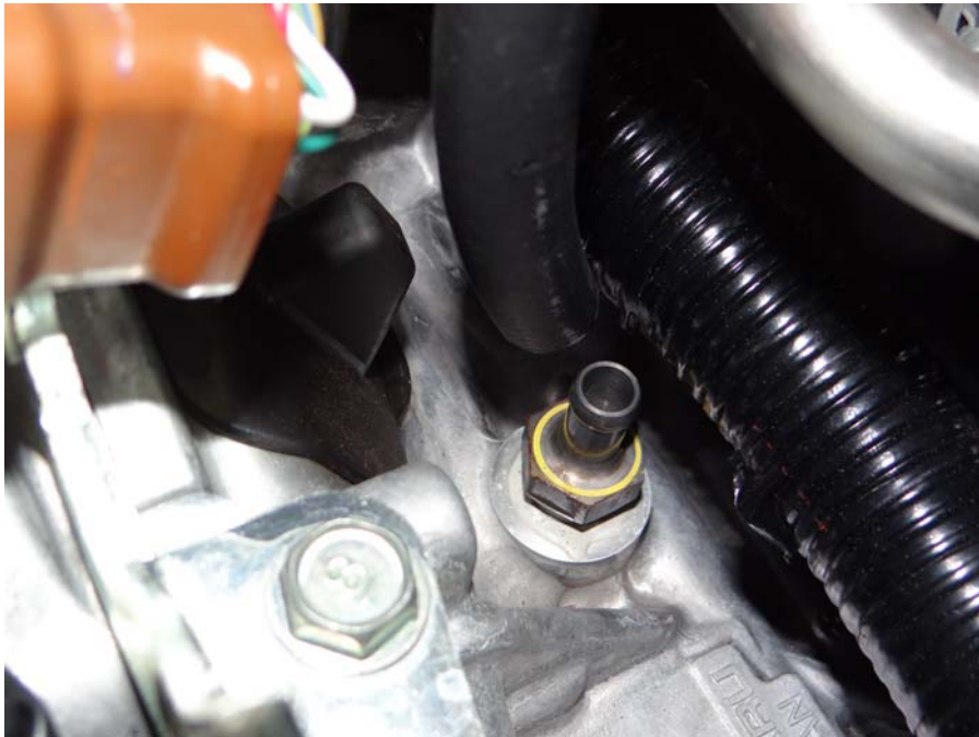
Step 5: Using length of 3/8" hose provided in kit, insert over crankcase nipple.
