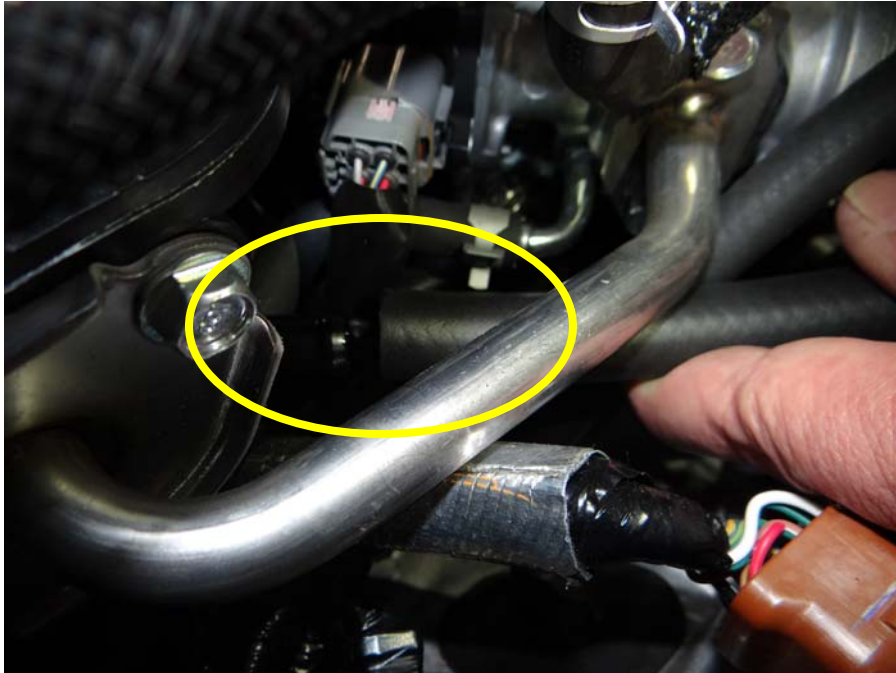
Step 6: Using length of ½” hose provided in kit, insert over intake nipple.
