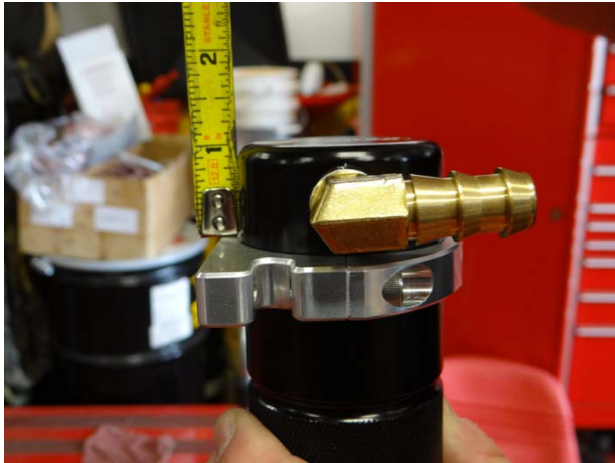
Step 12: Set height to 1"-1 1/8" and tighten billet clamp.
