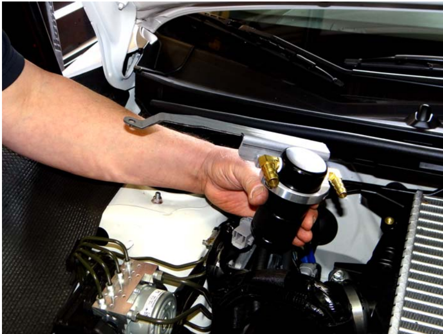
Step 15: Install Air Oil Separator assembly as shown in following illustrations.
