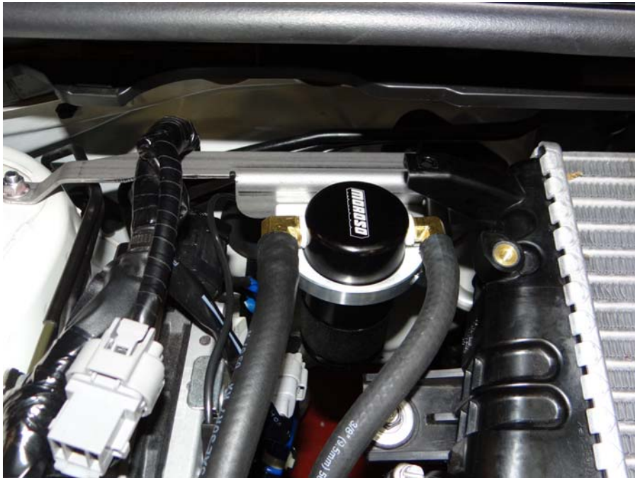
Step 16: Install hoses to Air Oil Separator, trimming of hoses will be required.
