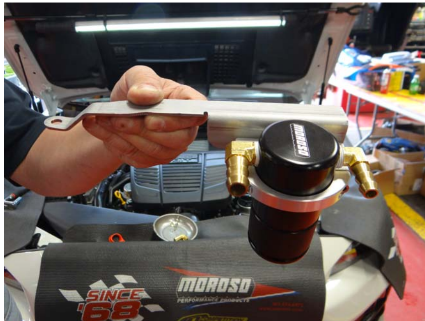
Step 13: Assemble Air Oil Separator to stainless steel mounting bracket as shown using (2) 1/4-20x5/8" SHCS.
