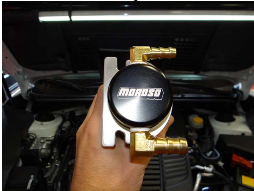
Step 11: With relief grooves facing down insert Air Oil Separator into billet clamp assembly.
