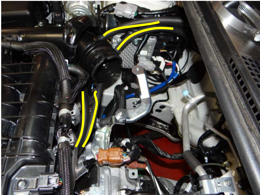
Step 7: Route hose as shown over to passenger's side of vehicle.
