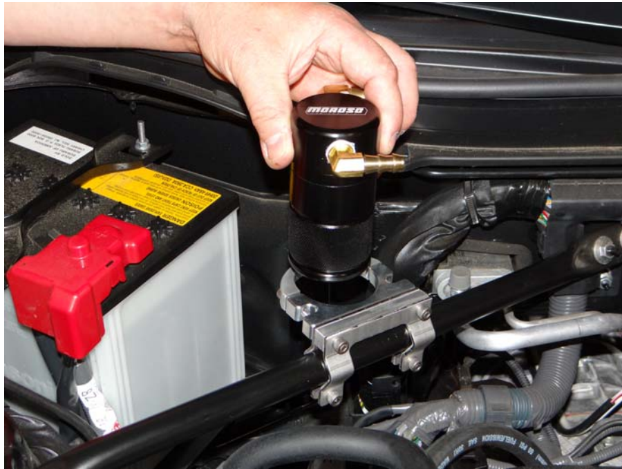
Step 11: Insert Air Oil separator into billet clamp.
